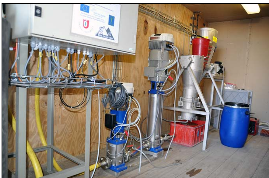
Figure 3.15. Mobile pilot unit for element extraction and recovery
