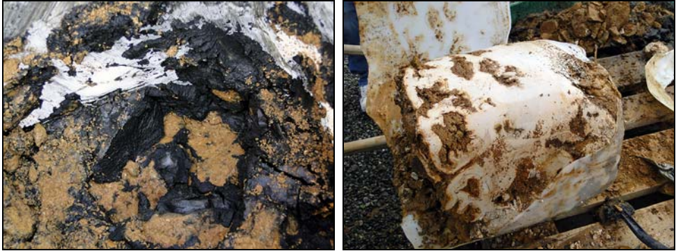
Figure 9.2. Injection with green liquor dregs (left) indicate, that all voids have been filled and that impermeable layers have been formed. Mine waste injected with lime kiln dust (right) has formed a solid unit with very low permeability
