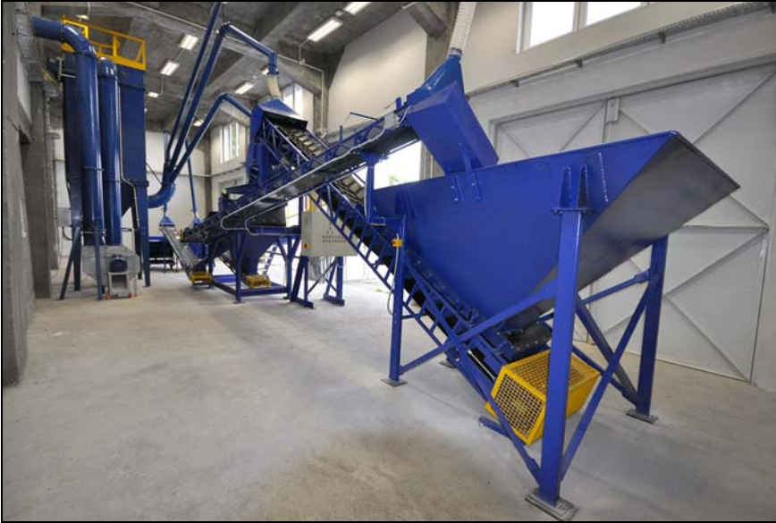
Figure 3.13. Installation for processing of wastes from coal processing plant
